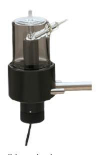
The Microcell is a dual purpose respirometer which can be used for flow through respirometry or alternatively for respiratory analysis of individually injected samples.
